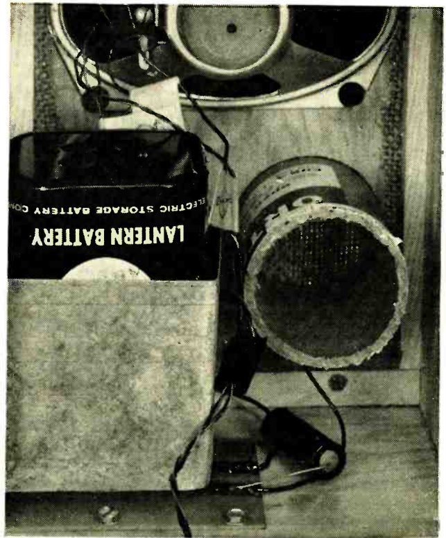
Ducted-port enclosures helps response from the 130-ohm center-tapped speakers designed for use with the CA3020 IC. PC contact board (beneath battery) insures correct polarity.
